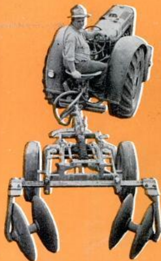
Cart equipped with hydraulic ram carries implements, controls bite into the soil
